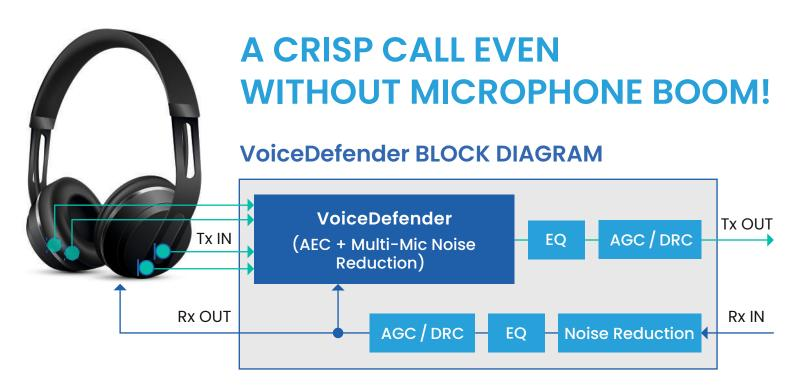
VoiceDefender employs adaptive directional beamforming on 4 microphone signals (2 per ear). A combination of end-fire and broadside beamforming is used to create a single enhanced output, providing a personal zone of voice preservation even in noisy environments.
